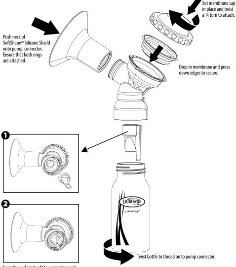
From the underside of the connector, push duckbill valve firmly onto the cylindrical piece inside the pump connector.
