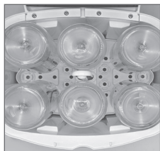
FIGURE E. Placement of wide-neck bottles
