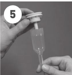
Snap the reservoir onto the insert.
